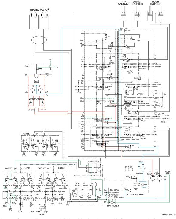
When the left control lever is pushed left or right, the swing spool in the main control valve is moved to the left or right swing position by the pilot oil pressure (PCs, PDs) from the remote control valve. Also the swing operation preference function is operated by the pilot pressure PCsp (refer to page 2-51).
