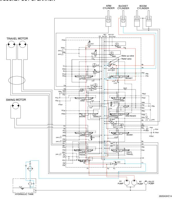
When the right control lever is pushed right, the bucket spool in the main control valve is moved to the roll out position by the pilot oil pressure (PBk) from the remote control valve.
