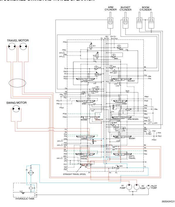
When the swing and travel functions are operated, simultaneously the swing spool and travel spools in the main control valve are moved to the functional position by the pilot oil pressure (PCs, PDs, PAtr, PBtr, PCtl, PDtl) from the remote control valve and straight travel spool is pushed to the right by the pilot oil pressure from the pilot pump.
