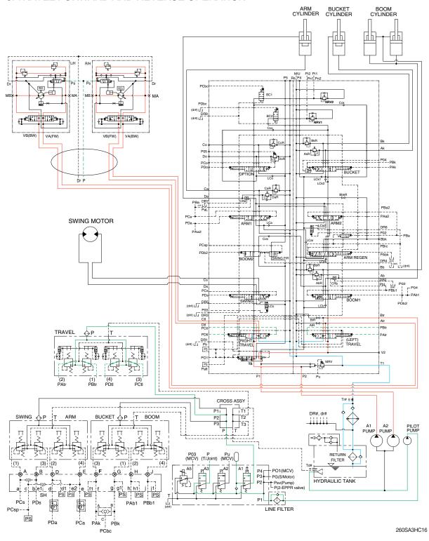
When the travel levers are pushed forward or reverse position, the travel spools in the main control valve are moved to the forward or reverse travel position by the pilot oil pressure (PAtr, PBtr, PCtl, PDtl) from the remote control valve.
