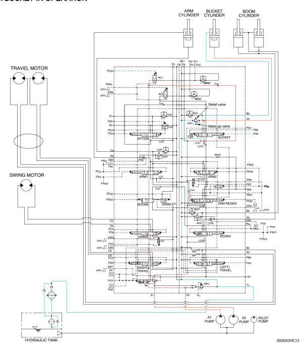
When the right control lever is pulled left, the bucket spool in the main control valve is moved to the roll in position by the pilot oil pressure (PAk) from the remote control valve.
