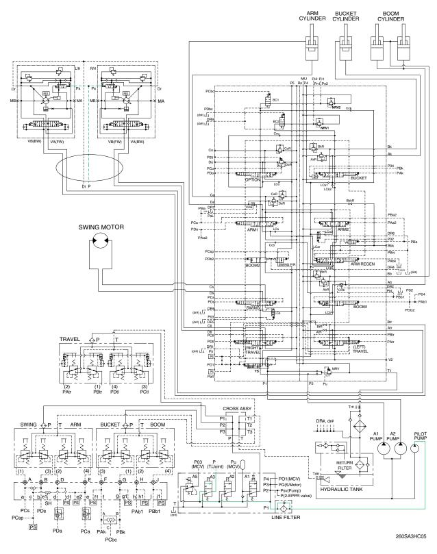
When the travel speed solenoid valve was placed in the Hi position, the pressure oil from pilot pump through line filter flows to port **Ps** of travel speed change over valve, and the control piston is pushed, thus minimizing the displacement.
