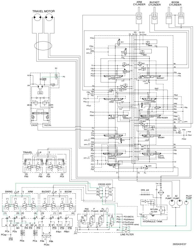
When the RCV lever (swing or arm in) is tilted, the pilot oil flows into SH port through shuttle valve. This pressure moves spool of the swing brake valve so, discharged oil from pilot valve flows to swing motor PG port. This pressure is applied to swing motor disc, thus the brake is released. When the RCV lever (swing and arm in) is set in the neutral position, oil in the swing motor disc cylinder is drained, thus the brake is applied.
